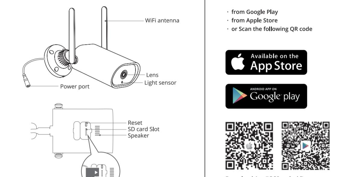
**CAUTION:** Please insert the Micro SD Card according to the direction shown in the diagram. Micro SD Card might be damaged if inserted incorrectly and device can be damaged.
